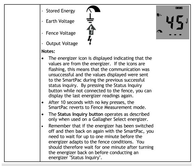
**Example of typical usage:** You noticed the fence load had increased on the energizer display. You then go out onto the farm to find the fault using your SmartPac and make the repair, (e.g. wire on the ground or damaged insulator). Once repaired, you then check, from the farm, that the fault you repaired put the energizer back to normal operation. This gives you confidence that the repair fixed the problem and there weren't additional faults.
