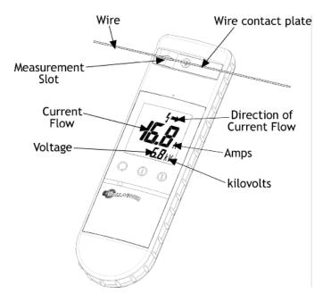
3. The Arrows on the display ( ( )) indicates the direction the current is flowing. The size of the arrow indicates the size of the current. The current is displayed in Amps.
