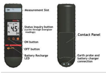
**IMPORTANT:** The SmartPac can communicate with a maximum of nine MX7500 or MR6000 energizers. For each energizer (MX7500 or MR6000) you want to communicate with, you need to complete the registrations process as described *Registration* (p 9).
